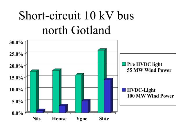
**Figure 3**. Voltage drop during obtained previous and after HVDC-Light connection during a short circuit in the AC network.
