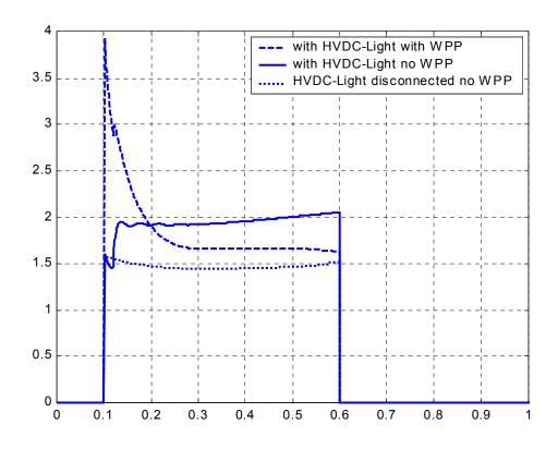
FIGURE 4. EFFECT OF HVDC-LIGHT AND WPP ON THE FAULT CURRENT DURING SHORT CIRCUIT AT NÄS
